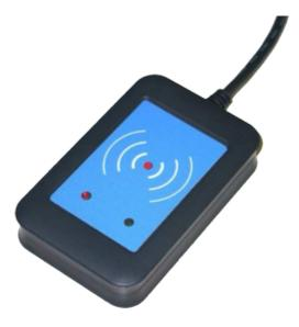
Key features of the TWN4 MultiTech 2 LF and HF desktop reader include a powerful SDK for writing apps that are executed directly on the reader, the possibility to upgrade the firmware in the field and a direct chip-commands support. Additionally, the reader can simultaneously read more than 60 RFID technologies from low (LF) and high frequency (HF) bands, including NFC. This gives the option to select as many of the technologies required instead of being forced to select just a few ones.
